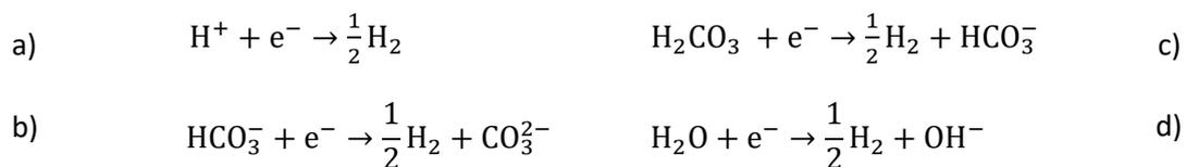
Reaction 2 Cathodic reactions for carbon steel in CO<sub>2</sub> aqueous solution. Only electrochemical reaction a) is considered in the buffering effect mechanism
