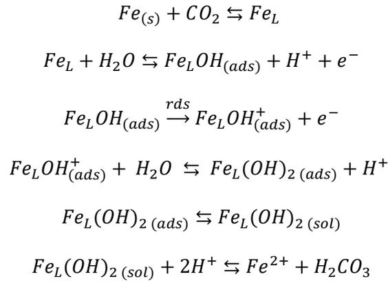
Reaction 5 Iron dissolution mechanism at pH>5 [28].
