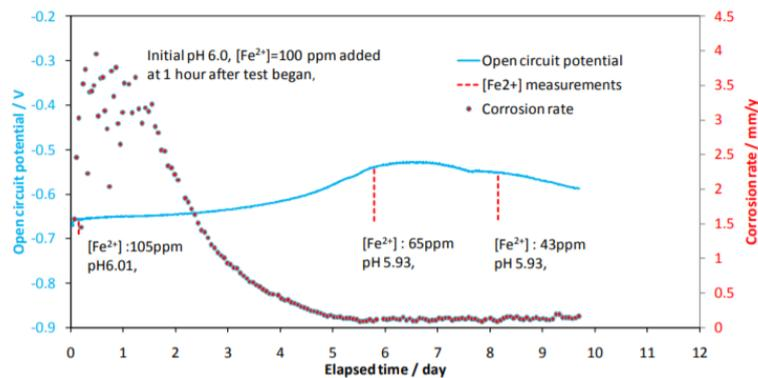
Figure 5 OCP variations and corrosion rate as function of exposure time at 80°C, pH 6.0, 0.53 bar [53 kPa] CO<sub>2</sub>, 1 wt% NaCl [48].
