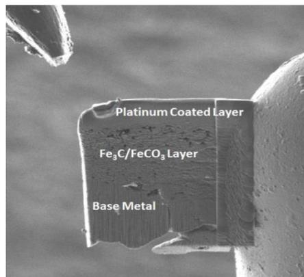
Figure 3 cross section TEM image of a of corrosion product on X65 steel on a CO<sub>2</sub> saturated 10 wt% NaCl at 80°C after 168 h [43].
