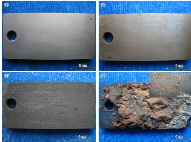
Figure 6 Photographs of corrosion product layer developed at 50°C CO<sub>2</sub>, 10 MPa, O<sub>2</sub>: 2000 ppmv, H<sub>2</sub>S: 2000 ppmv. (a) CO<sub>2</sub>; (b) CO<sub>2</sub>+ O<sub>2</sub>; (c) CO<sub>2</sub>+ H<sub>2</sub>S and (d) CO<sub>2</sub>+ O<sub>2</sub>+ H<sub>2</sub>S [77].
