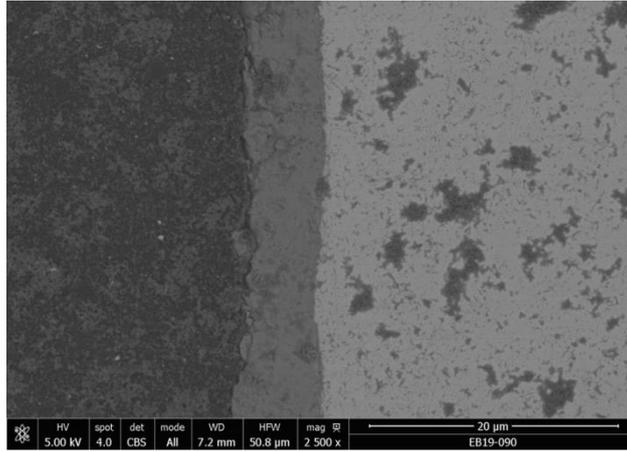
Figure 1 Cross section SEM micrograph of the corrosion product layer of a CO<sub>2</sub> saturate water solution at 80°C pH 6.8.
