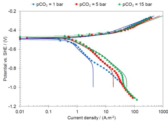
Figure 2 Polarizations curves on API 5L X65 mild steel at 10°C, 0.1 M NaCl, 4.4 m/s flow velocity, at pCO<sub>2</sub> of 1, 5, and 15 bar, at pH 6. Solid lines represent modeling with “buffer mechanism” [21].
