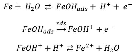
Reaction 4 Bockris anodic iron dissolution mechanisms [26,27].
