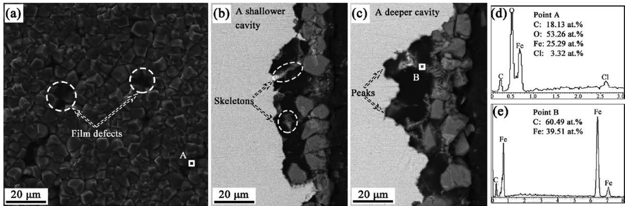
Figure 5 SEM micrographs (a) – (c) of morphologies of corrosion product layer for carbon steel in Cl-containing CO<sub>2</sub> saturated solution. (d) –(e) relative EDS analysis [62].
