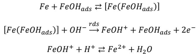
Reaction 3 Heusler anodic iron dissolution mechanism [25].
