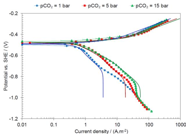
Figure 2 Polarizations curves on API 5L X65 mild steel at 10°C, 0.1 M NaCl, 4.4 m/s flow velocity, at pCO<sub>2</sub> of 1, 5, and 15 bar, at pH 6. Solid lines represent modeling with “buffer mechanism” [18].
