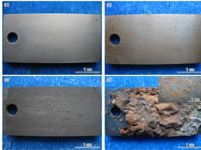
Figure 7 Photographs of corrosion product layer developed at 50°C CO<sub>2</sub>: 10 MPa, O<sub>2</sub>: 2000 ppmv, H<sub>2</sub>S: 2000 ppmv. (a) CO<sub>2</sub>; (b) CO<sub>2</sub>+ O<sub>2</sub>; (c) CO<sub>2</sub>+ H<sub>2</sub>S and (d) CO<sub>2</sub>+ O<sub>2</sub>+ H<sub>2</sub>S [77].
