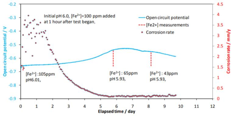
Figure 4 OCP variations and corrosion rate as function of exposure time at 80°C, pH 6.0, 0.53 bar 53 kPa CO<sub>2</sub>, 1 wt% NaCl [51].
