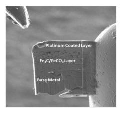
Figure 4 cross section TEM image of a of corrosion product on X65 steel on a CO2 saturated 10 wt% NaCl at 80°C after 168 h [40].
