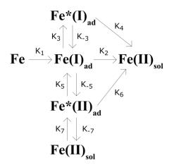
Figure 3 Keddam mechanism schema [23,24].
