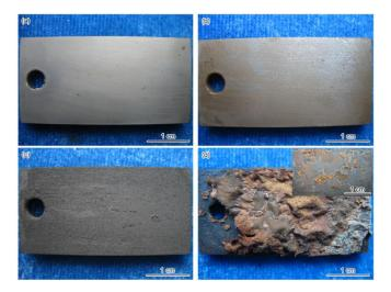
Figure 6 Photograps of corrosion product layer developed at 50°C CO2, 10 MPa, O2: 2000 ppmv, H2S: 2000 ppmv. (a) CO2; (b) CO2+ O2; (c) CO2+ H2S and (d) CO2+ O2+ H2S [77].
