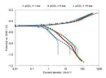
Figure 2 Polarizations curves on API 5L X65 mild steel at 10°C, 0.1 M NaCl, 4.4 m/s flow velocity, at pCO<sub>2</sub> of 1, 5, and 15 bar, at pH 6. Solid lines represent modeling with "buffer mechanism" [18].
