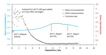
Figure 5 OCP variations and corrosion rate as function of exposure time at 80°C, pH 6.0, 0.53 bar [53 kPa] CO<sub>2</sub>, 1 wt% NaCl [48].
