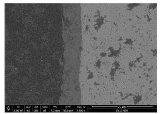
Figure 1 Cross section SEM micrograph of the corrosion product layer of a CO2 saturate water solutionat 80°C pH 6.8.
