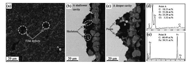
Figure 6 SEM micrographs (a) - (c) of morphologies of corrosion product layer for carbon steel in Cl<sup>-</sup> containing CO<sub>2</sub> saturated solution. (d) - (e) relative EDS analysis [57].
