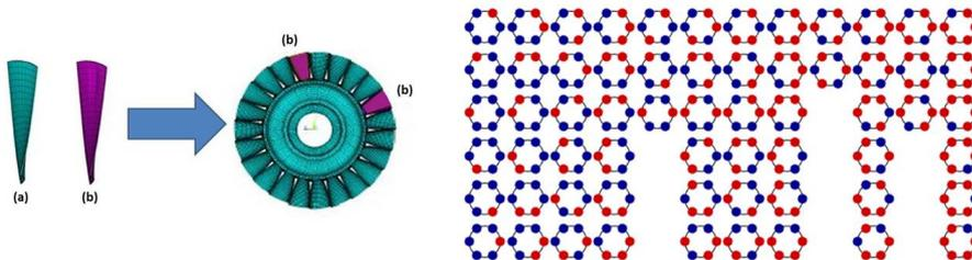
**Fig. 1** Left: A 23-blade configuration (from [34]) with two different pre-defined shapes (a) and (b). Right: the first line displays the twelve possible distinct 6-blade configurations (all equivalent variants, obtained by rotation, are listed column-wise)
