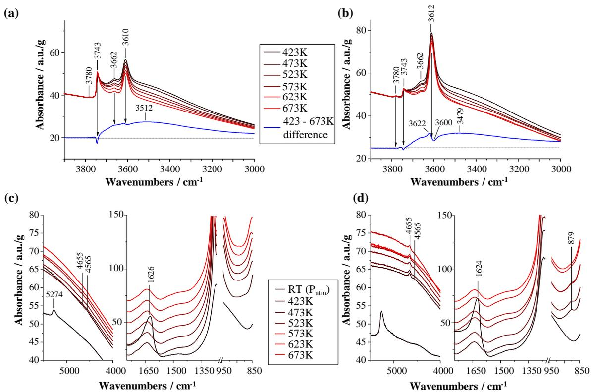
**Figure 4.** IR spectra of (a)-(c) Z-25-Small, (b)-(d) Z-22-Big, in the O-H stretching region (a)-(b), and in combination band plus bending zone (c)-(d). All spectra are acquired under secondary vacuum.
