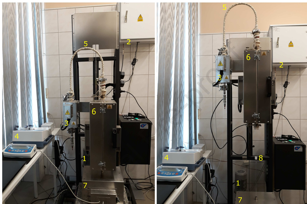
Fig. 1. Test rig for petcoke gasification in the gravimetric mode with the furnace in the lower (left) and upper (right) position (1 – electric motor, 2 – gaseous mixture preparation unit, 3 – evaporator, 4 – syringe pump, 5 – heated transfer line, 6 – the main furnace, 7 – weighing module, 8 – sample holder)
