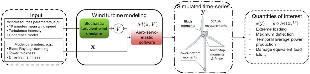
**FIGURE 1** General sketch for wind turbine modeling.
