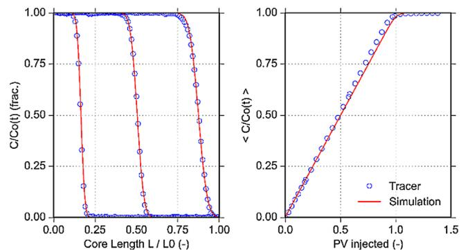
**Fig. 5.** Core dispersion fitted using a standard analytical solution [27]. The dispersion is fitted using the concentration profile monitored at 0.17 PV, 0.5 PV, 0.88 PV injected (left plot) and total tracer concentration (right plot). Dispersion is fitted to  $5.4 \times 10^{-9}$  m/s, corresponding to a dispersivity of 2 mm. Red lines show the simulated data, blue circles show the experimental data.
