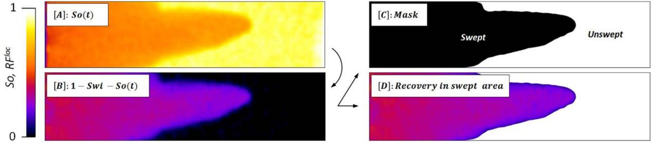
**Fig. 10.** CT-scan processing to compute the  $PV^{swept}$  and  $RF^{swept}$  values. (A) Shows the original saturation map, (B) shows the oil-recovery map compute as  $1 - Swi - So(t)$ , (C) shows the segmentation of the swept area and (D) shows the oil recovery in the swept area selection.
