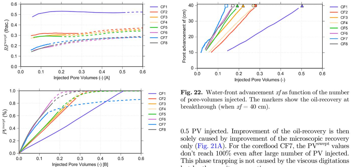
**Fig. 21.**  $PV^{\text{swept}}$  and  $Mic^{\text{rec}}$  values measured at BT on the 3D CT-scans, as function of the number of PV injected. Plain lines show the values before BT, dashed lines show the values after BT.
