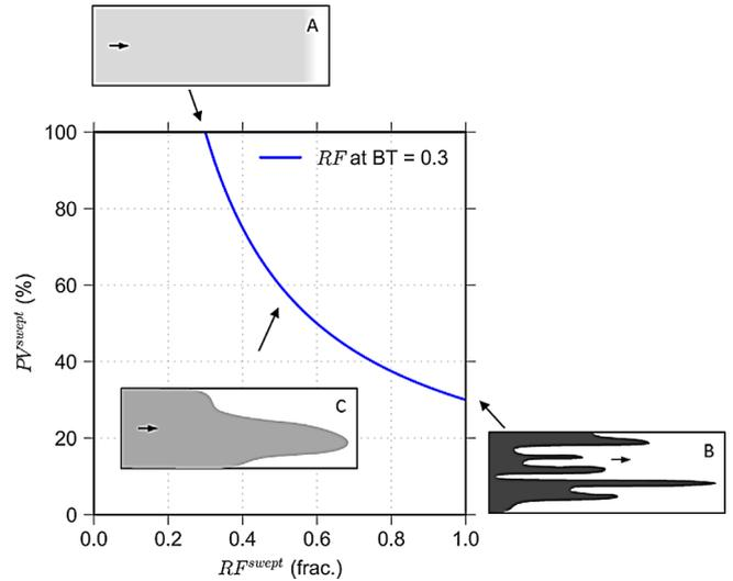
**Fig. 19.** Illustration of the digitation's characterization using the  $PV^{swept}$  and  $RF^{swept}$  values. Three possible digitations patterns A, B and C are shown resulting in the same RF at BT of 0.3. In this illustration, darker shades suggest higher water-saturation.
