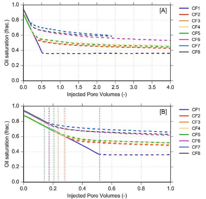
**Fig. 12.** Oil saturation monitoring of all corefloods (A), zoomed on the first injected pore volume (B). Plain lines show before BT, dashed lines are after BT (separation is indicated by the vertical dotted lines).
