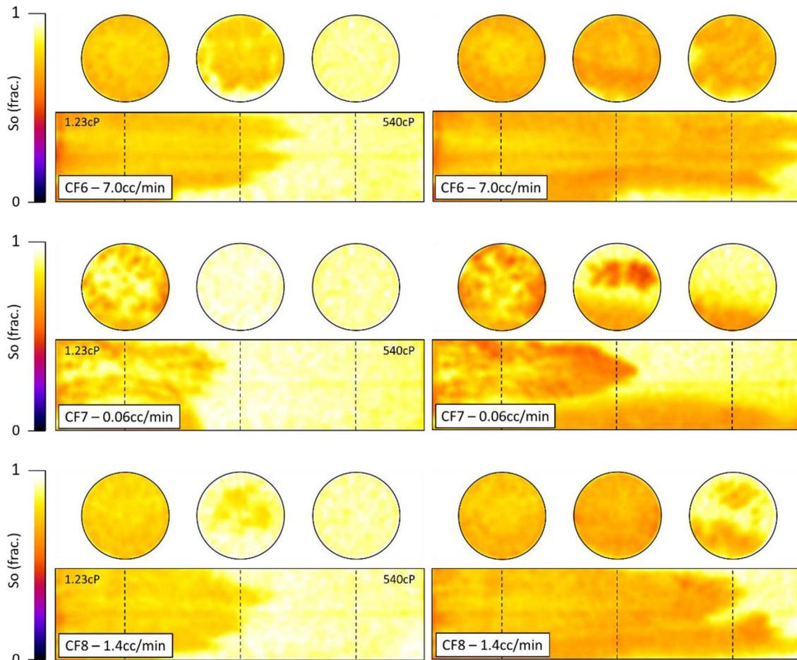
**Fig. 15.** 2D visualization of the front digitations using sagittal and transverse slices, for the oil-wet case after the core ageing (coreflood CF6–CF8). The displacement is displayed at half the breakthrough on the left and at breakthrough on the right. Positions of the transverse slices are marked by the dotted black lines. The sagittal slicing is illustrated [Figure 7](#).
