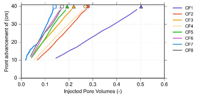
**Fig. 22.** Water-front advancement  $xf$  as function of the number of pore-volumes injected. The markers show the oil-recovery at breakthrough (when  $xf = 40$  cm).
