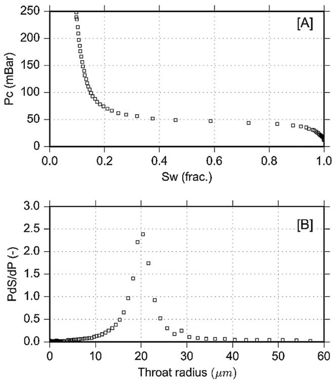
**Fig. 3.** Mercury intrusion capillary pressure measurement run on a twin Bentheimer sample. (A) Capillary pressure computed for our fluids and rock system, considering an IFT of 45 mN/m and a contact angle of 0 °C. (B) Throat radius distribution centered around 20 µm.
