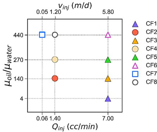
**Fig. 6.** Experimental corefloods design. Plain markers refer to corefloods conducted before the core ageing (water-wet case). Empty markers refer to corefloods conducted on the aged core (oil-wet). The injection velocity is computed as  $v_{inj} = Q_{inj}/(S^* \phi)$ , with  $S$  the core inlet surface.
