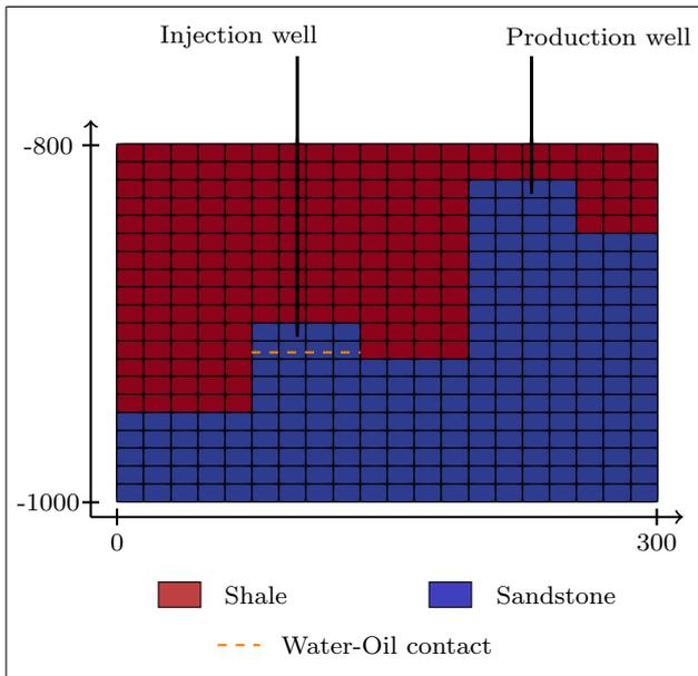
**Fig. 5** Second illustration case geometry, mesh and wells positions
