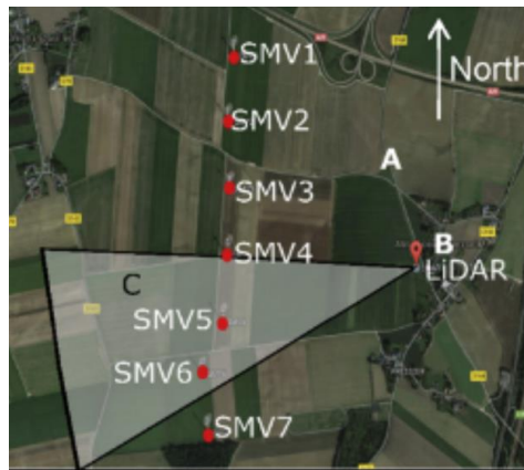
Figure 1: The wind farm composed of seven WTs marked with red dots. A meteorological mast (A) is located in the surrounding area. The location of the LiDAR is marked with B. The shadowed area, C, is the top view of the area scanned by the LiDAR [1].
