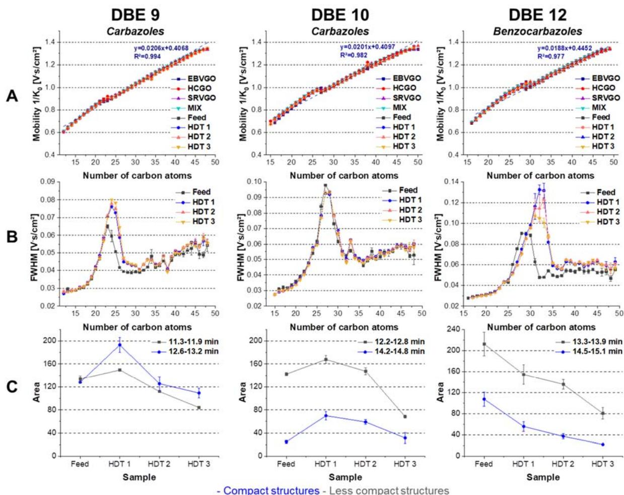
Figure 4: (A) Evolution of the mobility as a function of number of carbon atoms for the different DBE of all samples. (B) Evolution of the full-width at half-maximum (FWHM) as a function of number of carbon atoms for the different DBE of the feeds. (C) Evolution of the full-width at half-maximum (FWHM) as a function of number of carbon atoms for the different DBE of the hydrotreated samples.
