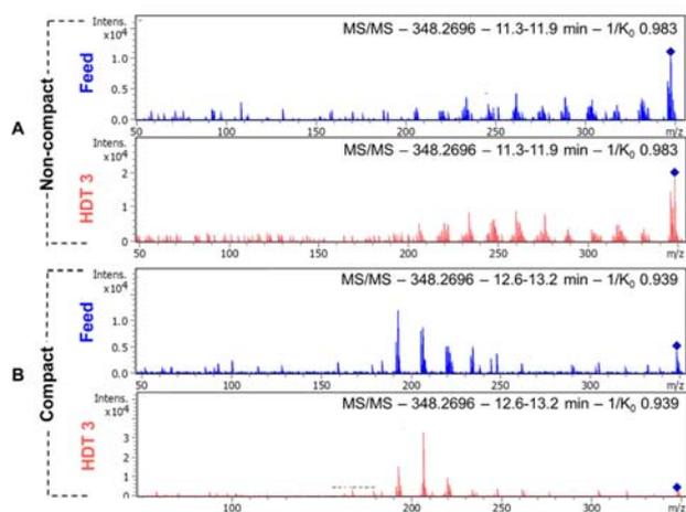
Figure 5: (A) Fragmentation spectra of  $C_{25}H_{35}N_1$  compound obtained for the feed and the sample HDT 3 in non-compact configuration. (B) Fragmentation spectra obtained for the feed and the sample HDT 3 in compact configuration.
