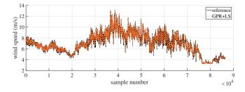
Fig. 5. Estimation for consecutive points to simulate a realtime application. The parameters are C = 5, r = 20,  $N = 10^4$ , and  $M = 3 \times 10^3$ . We use only the nearest cluster estimate.
