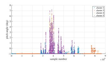
Fig. 3. Pitch angle time-series corresponding to Fig. 5. The points are color coded according to the cluster used for the estimation of the wind speed at the corresponding time.
