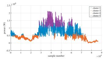
Fig. 4. Produced power time-series corresponding to Fig.5. The points are color coded according to the cluster used for the estimation of the wind speed at the corresponding time.
