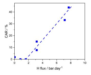
Figure 7: Correlation between CAR and hydrogen diffusion flux.
