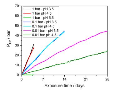
Figure 5: Time evolution of hydrogen pressure in the cavity of X70 hollow sensors exposed to aqueous test solutions at various pH and P<sub>H2S</sub>.
