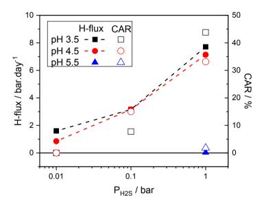
Figure 6: Evolution of hydrogen fluxes and CAR with P<sub>H2S</sub>.
