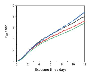
Figure 8: Time evolution of hydrogen pressure in the cavity of pure iron hollow sensors exposed to a test solution of pH 4.5, with 9.9 bar CO<sub>2</sub> and 0.1 bar H<sub>2</sub>S.
