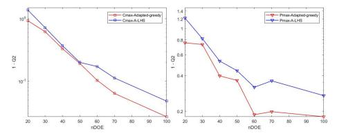
Figure 1: Accuracy of the surrogate models of the maximal torque (left) and the maximal power (right) built with designs of experiments obtained by the projected LHS method (in blue) and by the Adapted-Greedy algorithm (in red) with respect to the size of the designs.
