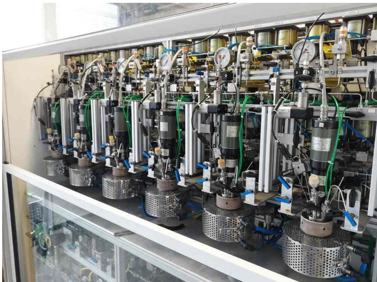
Figure S19 – Equipment used for catalyst screening consisting of 6 parallelized 100mL reactor (www.top-industrie.com).
