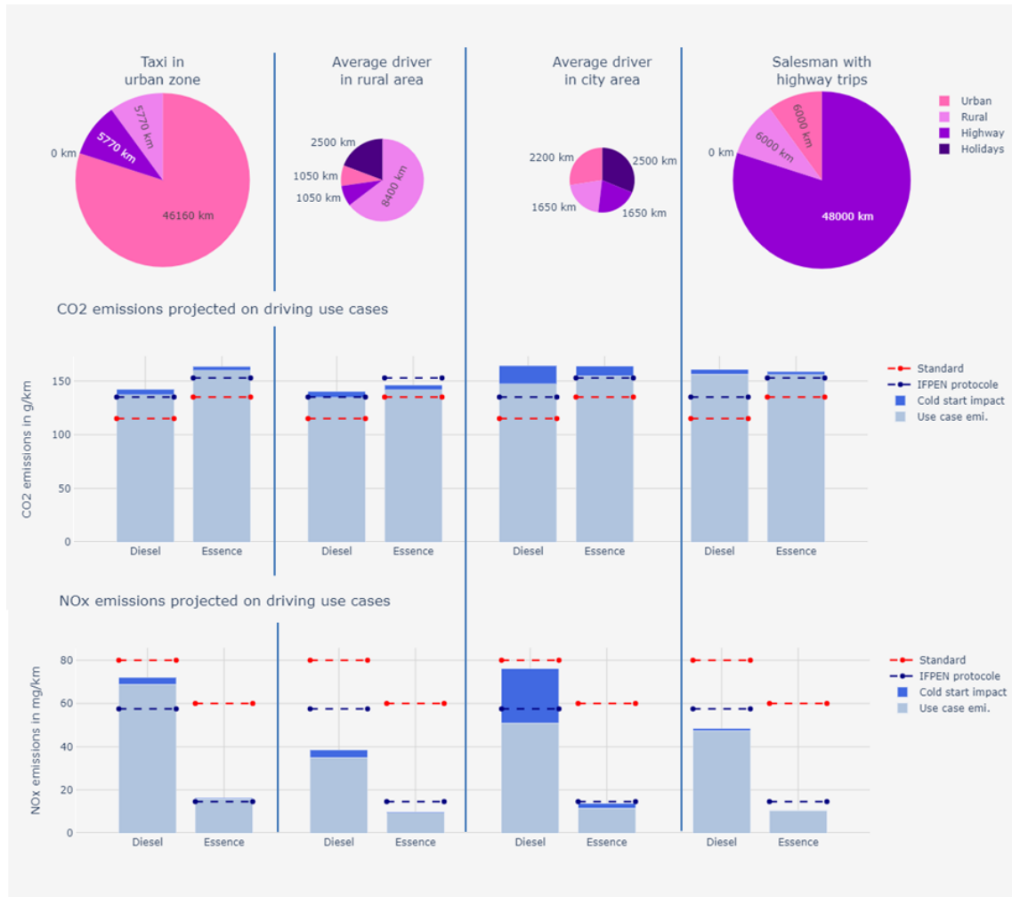
Figure 30 : Comparison of CO 2 and NO x emissions projected on uses for gasoline and diesel compact SUV vehicles (GV3 and DV3)
