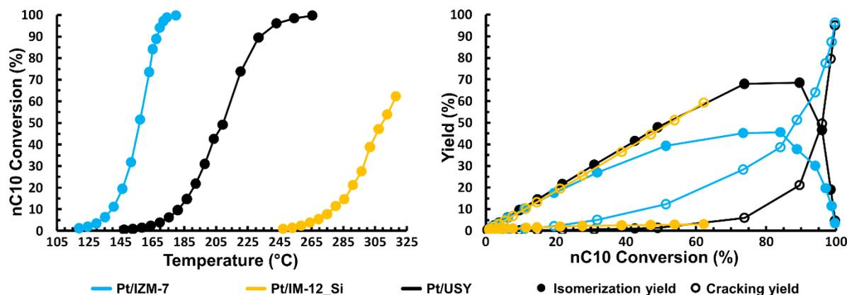
**Figure 3:** (a) Conversion of n-decane against reaction temperature, (b) yield of n-decane skeletal isomers and cracked products against n-decane conversion, of the 0.3 wt.% Pt/IM-12\_Si, 0.3 wt.% Pt/IZM-7 and 0.5wt.%Pt/USY catalysts.
