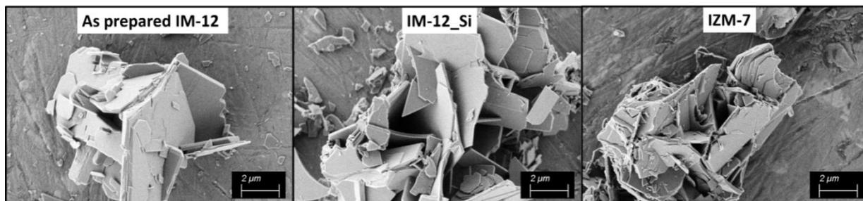
**Figure 2: SEM images of as prepared IM-12, IM-12 treated with SiCl<sub>4</sub> (IM-12\_Si) and IZM-7.**
