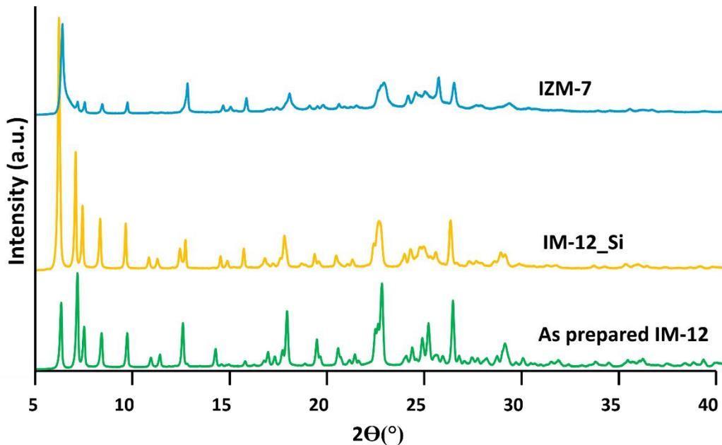
**Figure 1: XRD patterns of as prepared IM-12, IM-12 treated with SiCl<sub>4</sub> (IM-12\_Si) and IZM-7.**
