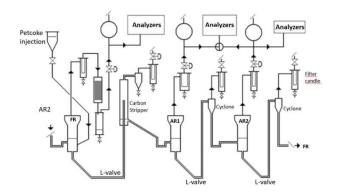
Figure 3: schematic view of IFPEN's 10 kW<sub>th</sub> unit
