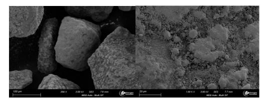
Figure 11: SEM images of LY-Mn ore powder after 52 hours of methane activation
