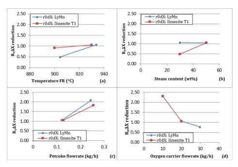
Figure 9: Evolution of  $R_0\Delta X$  with: (a) temperature of FR, (b) steam content, (c) petcoke flowrate, (d) oxygen carrier flowrate for Ilmenite T1 and LY Mn ore
