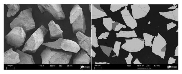
Figure 14: SEM images of ilmenite T1 (left: direct observation; right: polished cross-section)
