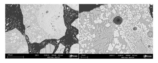
Figure 10: Cross-section SEM images of fresh LY-Mn ore
