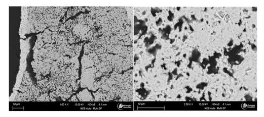
Figure 12: cross-section SEM images of LY-Mn ore powder after 52 hours of methane activation
