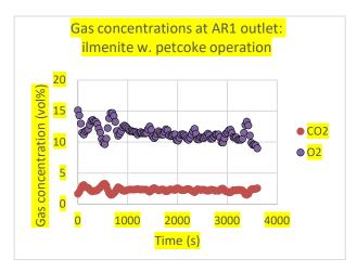
Figure 6: Profiles of gas concentrations at outlet of FR and AR1 during a reference test with solid fuel and Ilmenite as OC
