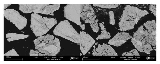
Figure 15: SEM cross-section analysis of Ilmenite during methane activation (left: after 34h; right: after 108h)
