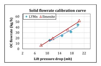
Figure 4 : Calibration curve of the solid flow rate in the unit over the pressure drop in the lift after AR2
