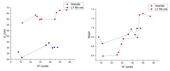
Figure 5: Evolution of methane conversion and RoDX during LY Mn ore activation cycles in comparison to Ilmenite T1 behavior
