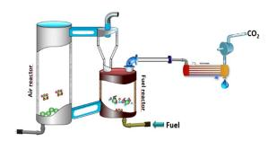
Figure 1: Diagram of chemical looping combustion process
