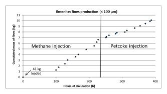
Figure 17: Mass of fines recovered as a function of circulation time during ilmenite campaign (Petcoke combustion was not performed on a continuous basis)
