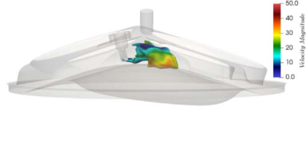
Fig. 7. Flame kernel development identified by the progress variable iso-surface at 0.5 coloured by the local velocity magnitude. Upper figure: fast burning cycle. Lower figure: slow burning cycle.
