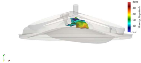
Fig. 7. Flame kernel development identified by the progress variable iso-surface at 0.5 coloured by the local velocity magnitude. Upper figure: fast burning cycle. Lower figure: slow burning cycle.
