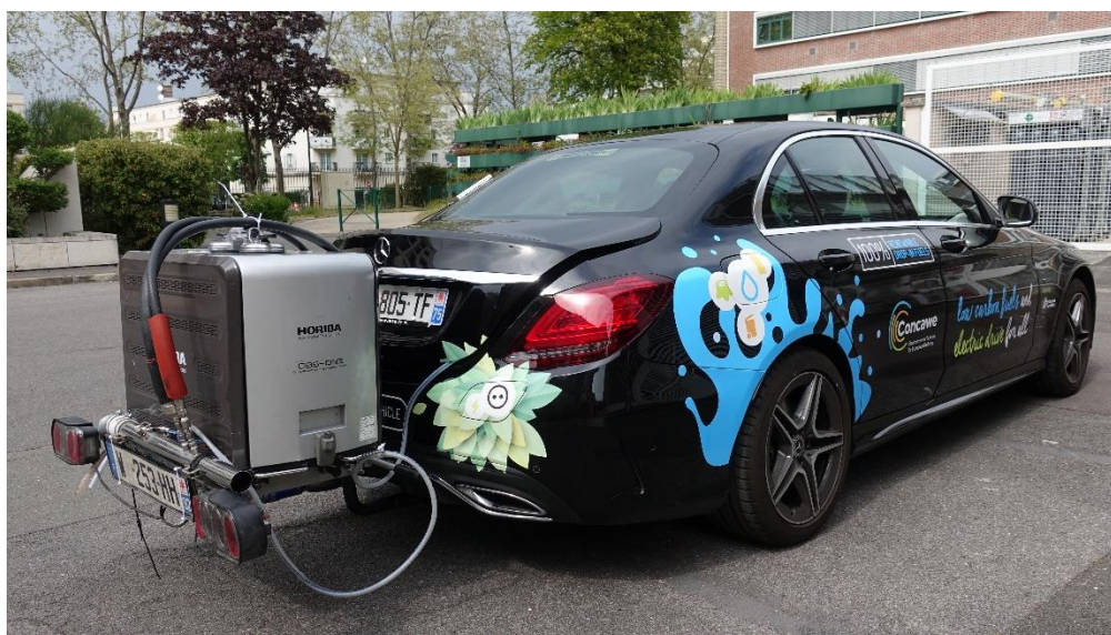
Figure 39 Vehicle setup for on-road tests, with PEMS equipment
