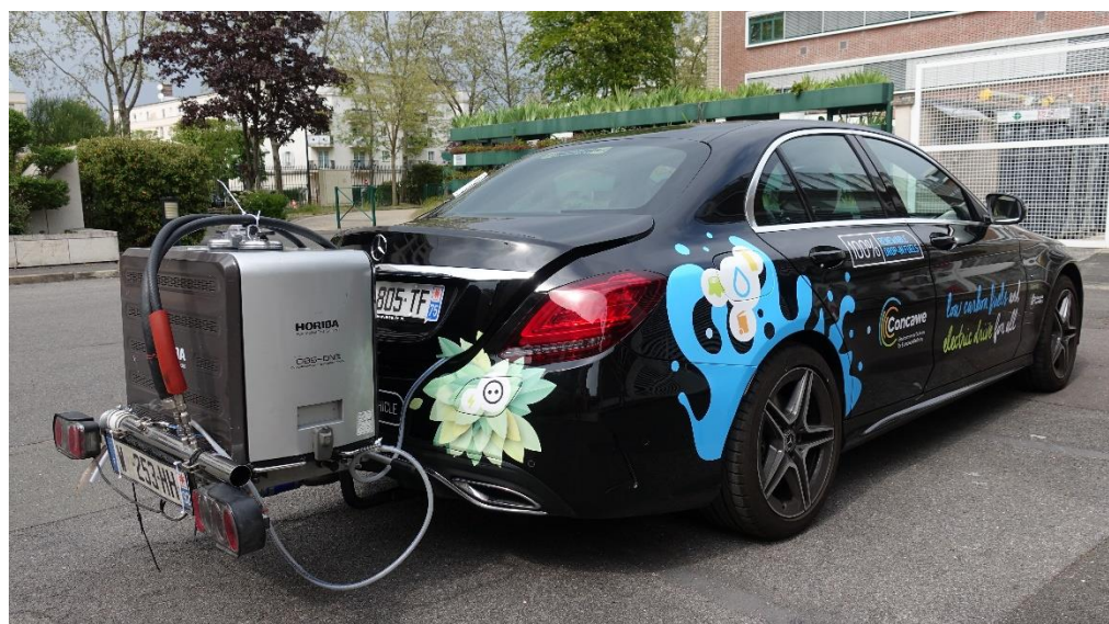
Figure 39 Vehicle setup for on-road tests, with PEMS equipment
