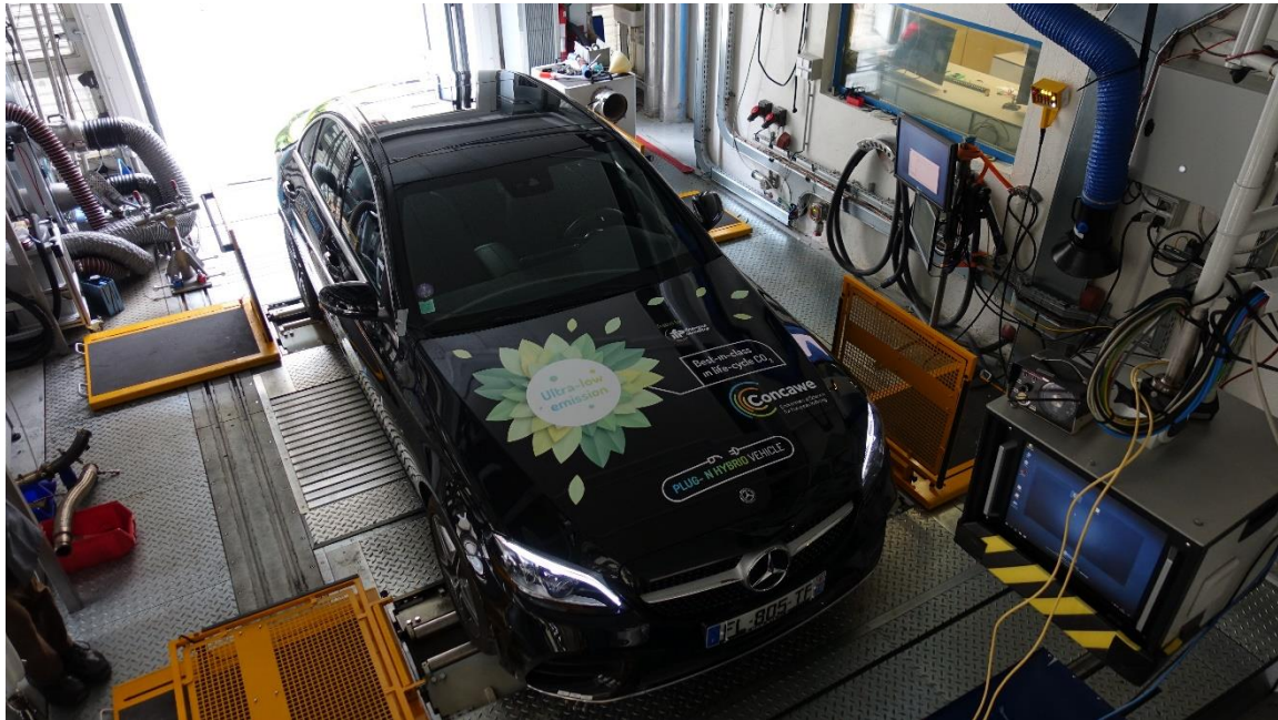
Figure 2 Picture of the chassis dyno setup with the tested vehicle
