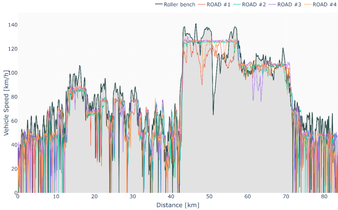
Figure 40 Vehicle speed profiles measured during on-road tests compared to the RDE cycle performed on the chassis dyno
