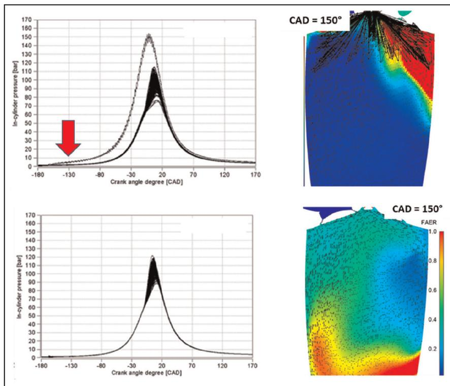
**Figure 2.** Impact of fuel distribution on occurrence of pre-ignition, 2000 rpm, mid load, lambda = 2. Reproduction from Duffour et al.<sup>45</sup>
