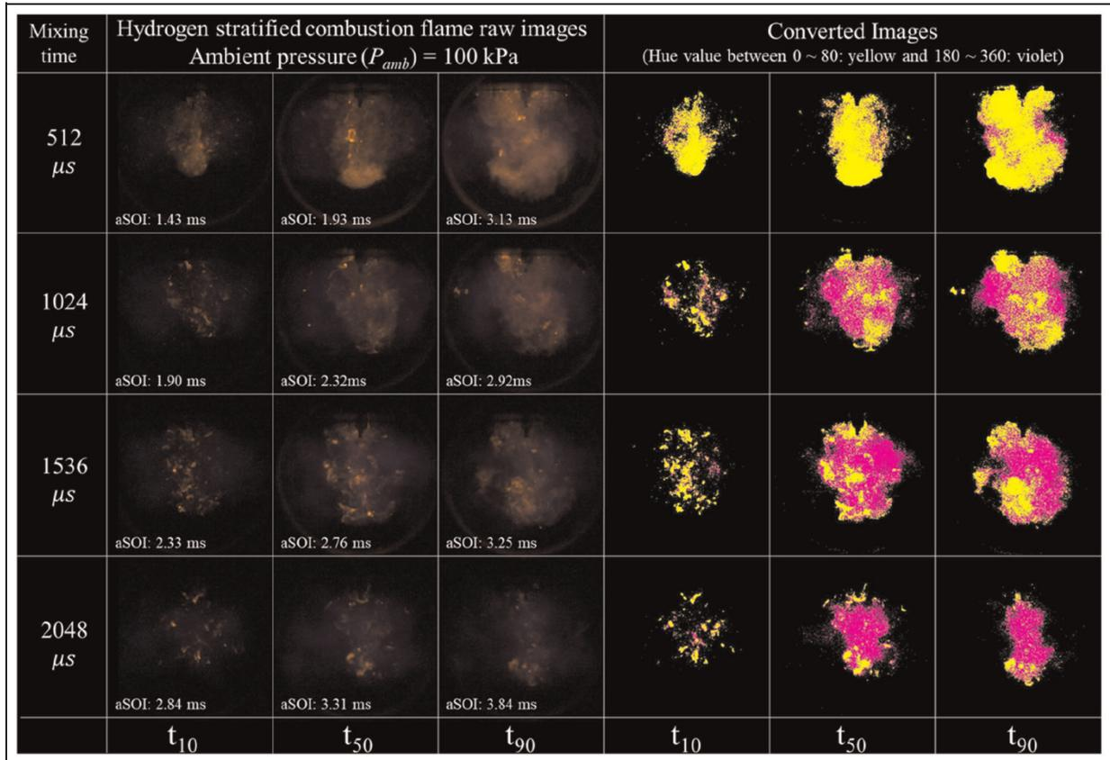
**Figure 4.** Direct flame images and Hue-based flame division converted images at different mixture formation times. Figure adapted from Lee et al.<sup>51</sup>
