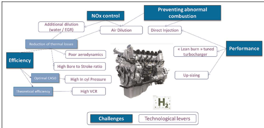
**Figure 1.** Technological assembly with respect to key challenges. Reproduction from Duffour et al.<sup>45</sup>
