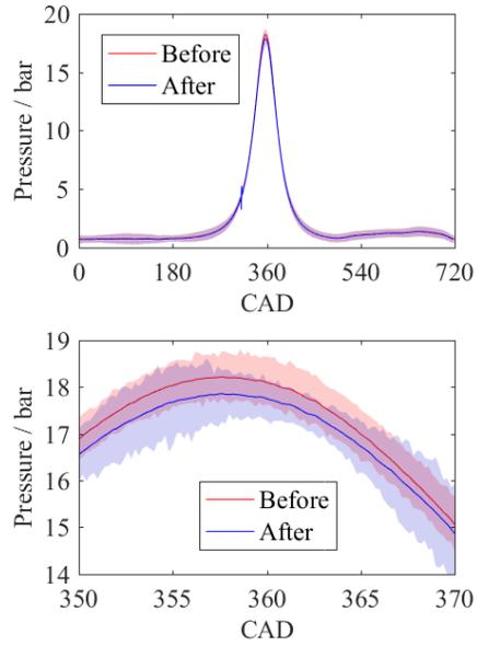
Figure 7: Pressure trace before and after dismounting and cleaning the optical engine under motored operation. Bottom: enlargement around TDC. Transparent overlay: variation in pressure from 500 consecutive cycles. The mean pressure traces are shown with a solid line.
