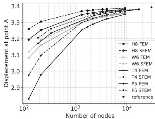
**FIGURE 25** Results for test case of Figure 19. Comparison between the values of the displacement of point A in Figure 19 obtained from the FS-FEM and FEM models for meshes of different element type and different element size ( $\alpha_{ir} = 0$ ). A reference solution from Reference 10 is shown as well.
