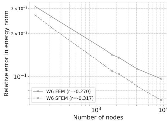
**FIGURE 34** Results for test case of Figure 19. Relative error in energy norm as defined in Equation (73) for the S-FEM and FEM numerical solutions for different element sizes for W6 meshes ( $\alpha_{ir} = 0.7$ )
