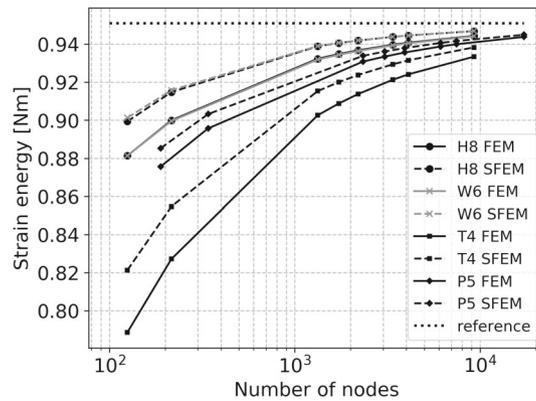
**FIGURE 26** Results for test case of Figure 19. Comparison between the values of the strain energy obtained from the FS-FEM and FEM models for meshes of different element type and different element size ( $\alpha_{ir} = 0$ ). A reference solution from Reference 10 is shown as well.
