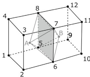
**FIGURE 2** Example of construction of a smoothing domain for FS-FEM method. The smoothing domain is built on the face defined by nodes 5, 6, 7, and 8 shared between the two hexahedral elements by connecting these four nodes with the element centroids A and B.
