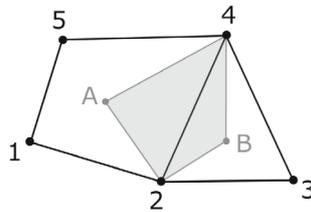
**FIGURE 1** Example of construction of a smoothing domain for ES-FEM method. The smoothing domain is built on the edge defined by nodes 2 and 4 shared between the quadrangular and triangular elements by connecting these two nodes with the element centroids A and B.
