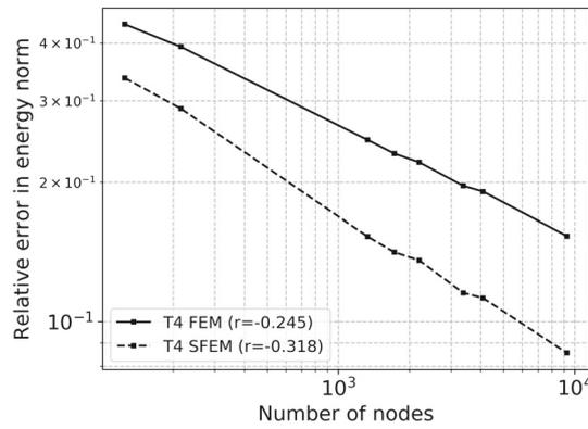
**FIGURE 35** Results for test case of Figure 19. Relative error in energy norm as defined in Equation (73) for the S-FEM and FEM numerical solutions for different element sizes for T4 meshes ( $\alpha_{ir} = 0.7$ )
