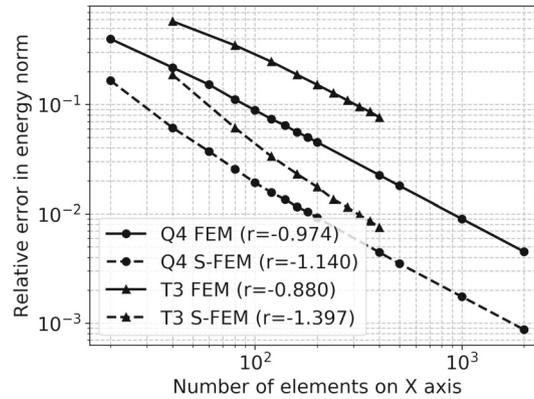
**FIGURE 18** Results for test case of Figure 11. Relative error in energy norm as defined in Equation (73) for the S-FEM and FEM numerical solutions for different element sizes for T3 and Q4 meshes ( $\alpha_{ir} = 0.7$ )
