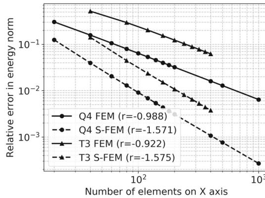
FIGURE 16 Results for test case of Figure 11. Relative error in energy norm as defined in Equation (73) for the S-FEM and FEM numerical solutions for different element sizes for T3 and Q4 meshes ( $\alpha_{ir} = 0$ )
