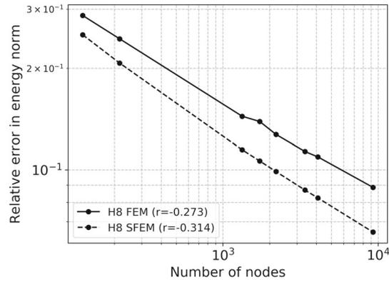
**FIGURE 27** Results for test case of Figure 19. Relative error in energy norm as defined in Equation (73) for the S-FEM and FEM numerical solutions for different element sizes for H8 meshes ( $\alpha_{ir} = 0.0$ )
