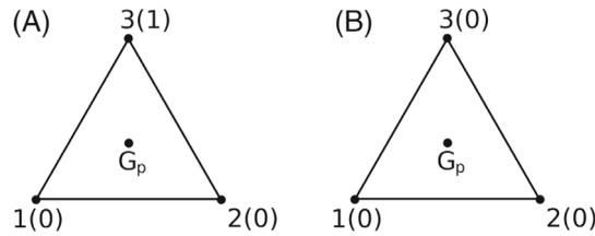
**FIGURE 7** Value of the shape functions at the nodes of a triangular base face of a smoothing domain (example of face 1-2-3 in Figure 4). The numbers in parenthesis near the node label are the value of the shape function at the node.  $G_p$  is the centroid of the face. (A) Example of the values when the shape function is associated to a node of the face ( $N_3(\mathbf{x})$  in the figure). (B) Example of the values when the shape function is not associated to a node of the face.
