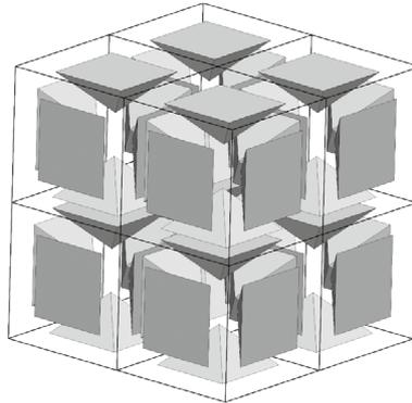
**FIGURE 23** Example of the mesh of uniform pyramidal elements obtained by splitting the hexahedral mesh of Figure 20. Wireframe view of hexahedral mesh of Figure 20 is shown. Pyramidal elements are shrunk to show how they have been obtained from hexahedral elements.
