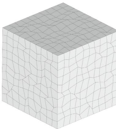
**FIGURE 24** Example of a distorted H8 mesh ( $\alpha_{ir} = 0.7$ )
