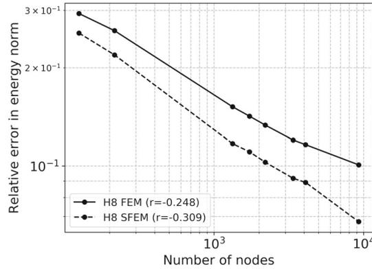
**FIGURE 33** Results for test case of Figure 19. Relative error in energy norm as defined in Equation (73) for the S-FEM and FEM numerical solutions for different element sizes for H8 meshes ( $\alpha_{ir} = 0.7$ )
