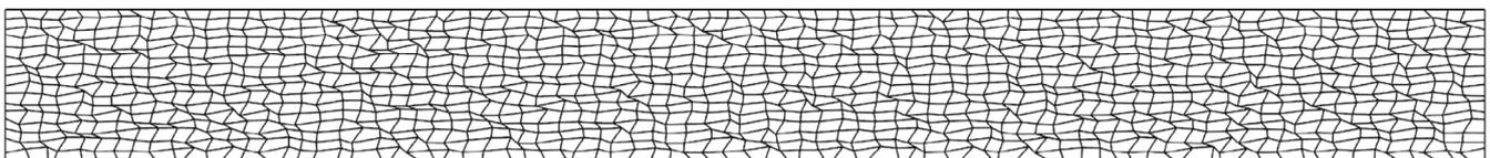
**FIGURE 13** Example of a distorted Q4 mesh ( $\alpha_{ir} = 0.7$ )
