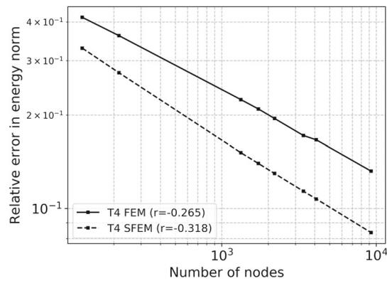
**FIGURE 29** Results for test case of Figure 19. Relative error in energy norm as defined in Equation (73) for the S-FEM and FEM numerical solutions for different element sizes for T4 meshes ( $\alpha_{ir} = 0.0$ )
