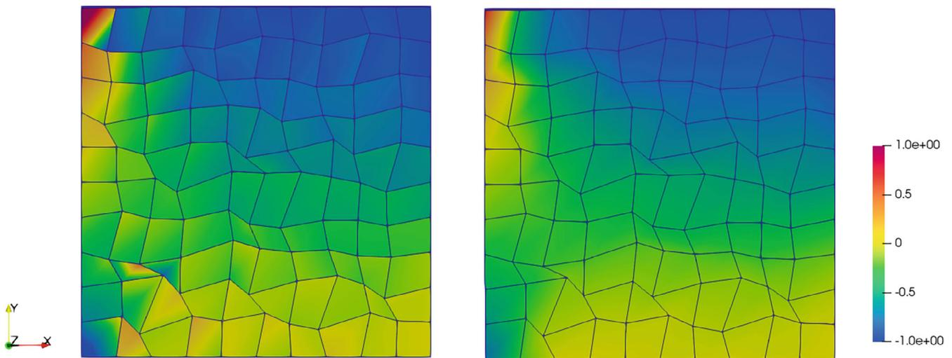
**FIGURE 37** Effect of the change in the sign of the Jacobian on the FEM stress field,  $\sigma_y$ , stress component (Pa) for the external face at  $z = 0.5$  of the cube of Figure 19. The H8 mesh is distorted with an irregularity factor  $\alpha_{ir} = 0.7$ . On the left: FEM solution. On the right: FS-FEM solution
