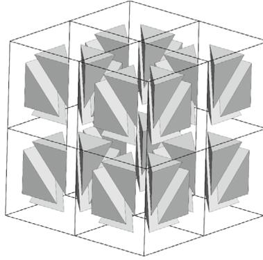
**FIGURE 22** Example of the mesh of uniform tetrahedral elements obtained by splitting the hexahedral mesh of Figure 20. Wireframe view of hexahedral mesh of Figure 20 is shown. Tetrahedral elements are shrunk to show how they have been obtained from hexahedral elements.
