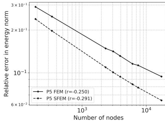
FIGURE 30 Results for test case of Figure 19. Relative error in energy norm as defined in Equation (73) for the S-FEM and FEM numerical solutions for different element sizes for P5 meshes ( $\alpha_{ir} = 0.0$ )
