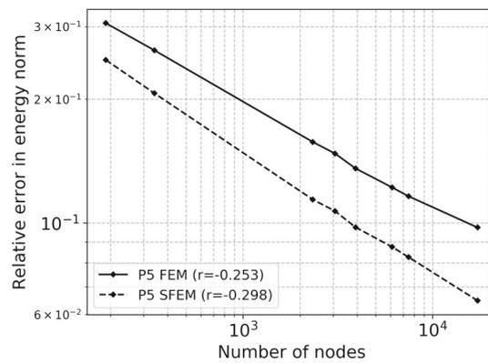
**FIGURE 36** Results for test case of Figure 19. Relative error in energy norm as defined in Equation (73) for the S-FEM and FEM numerical solutions for different element sizes for P5 meshes ( $\alpha_{ir} = 0.7$ )
