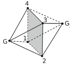
**FIGURE 5** Example of smoothing domain generated by a quadrangular face (face 1-2-3-4). Points G and G<sup>1</sup> are the centroids of the two elements sharing face 1-2-3. The smoothing domain is composed by the two pyramids 1-2-3-4-G and 1-2-3-4-G<sup>1</sup>.
