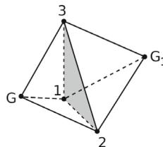
**FIGURE 4** Example of smoothing domain generated by a triangular face (face 1-2-3). Points G and G<sup>1</sup> are the centroids of the two elements sharing face 1-2-3. The smoothing domain is composed by the two tetrahedra 1-2-3-G and 1-2-3-G<sup>1</sup>.
