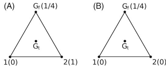
**FIGURE 9** Value of the shape functions at the one of the four triangles used to split the quadrangular face in Figure 8. The numbers in parenthesis near the node label are the value of the shape function at the node/point.  $G_f$  is the centroid of the quadrangular face. (A) Example of the values when the shape function is associated to a node of the face ( $N_2(\mathbf{x})$  in the figure). (B) Example of the values when the shape function is not associated to a node of the face.
