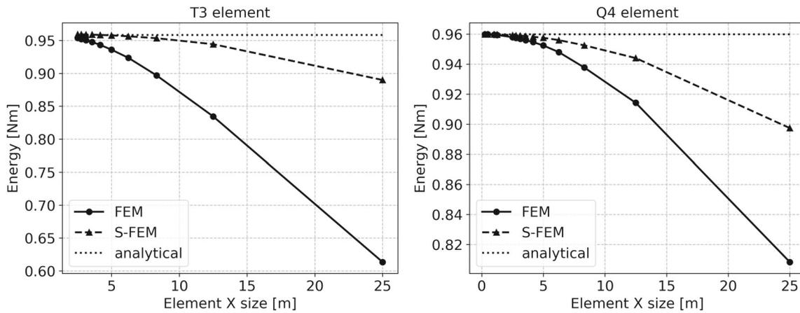
**FIGURE 17** Results for test case of Figure 11. Comparison between the elastic strain energy obtained from S-FEM and FEM models for different element sizes and the value from the analytical solution for T3 and Q4 meshes ( $\alpha_{ir} = 0.7$ )
