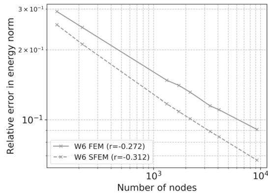
**FIGURE 28** Results for test case of Figure 19. Relative error in energy norm as defined in Equation (73) for the S-FEM and FEM numerical solutions for different element sizes for W6 meshes ( $\alpha_{ir} = 0.0$ )
