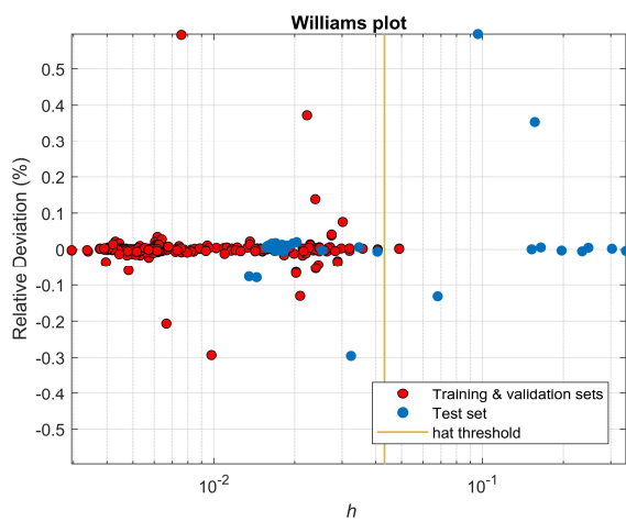
Figure S21. Williams plot for the density data of the (water + NaF) system.
