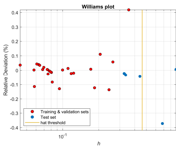
Figure S23. Williams plot for the density data of the (water + RbF) system.
