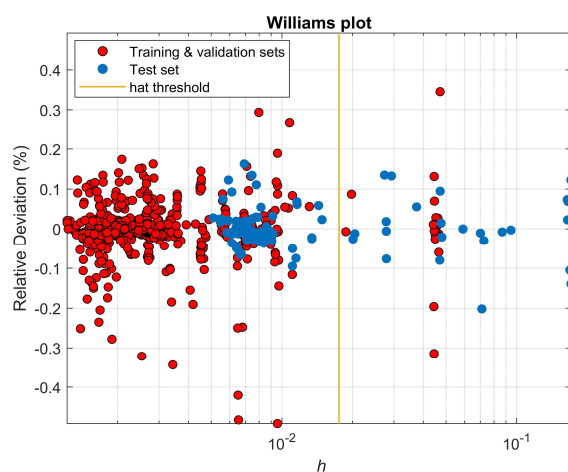
Figure S31. Williams plot for the density data of the (water + KBr) system.
