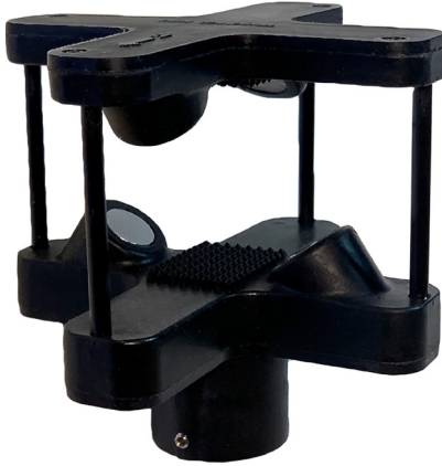
Figure 2. TriSonica Mini Wind Sensor is the World's smallest ( 91 \times 91 \times 52 mm) and lightest (50 grams) low velocity (less than 50 m/s) ultrasonic anemometer with a maximum data output rate of 60 Hz.
