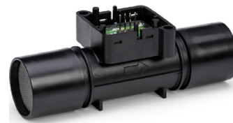
Figure 3. SFM3000 from Sensirion AG is a bi-directional hot-wire anemometer, which is compact ( 82 \times 35 \times 32 mm), lightweight (17 grams) and high data output rate (up to 2 kHz).
