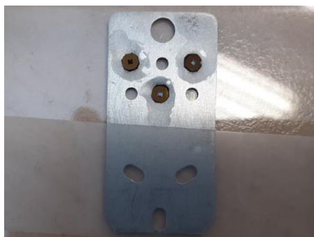
Figure S.3: Sample holder with glued TEM grid.
