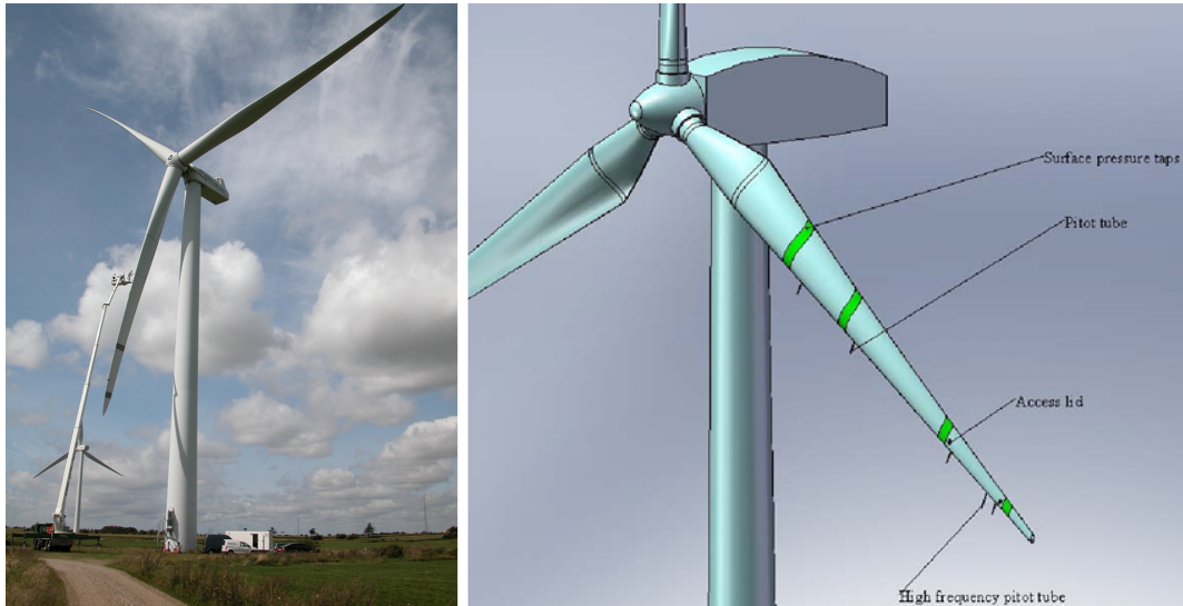
Figure 1. DanAero turbine and instrumentation (Bak et al., 2010).
