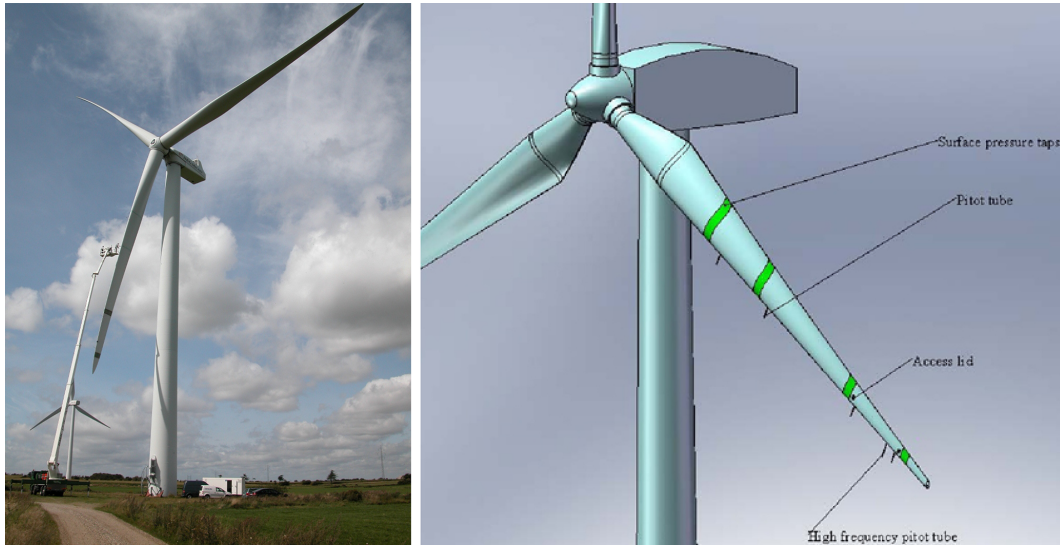
Figure 1. DanAero turbine and instrumentation (Bak et al., 2010).
