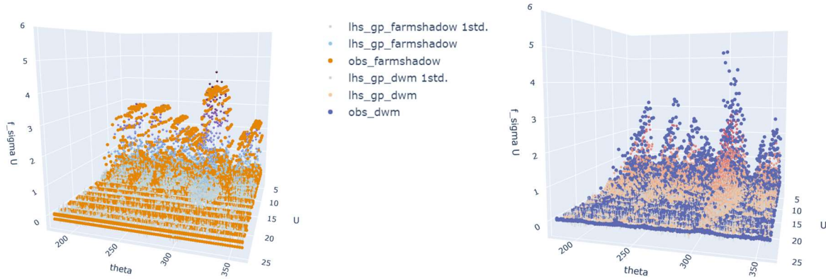
Figure 84 : Teesside: GP prediction of the f_{\sigma_u} for a large LHS. Error bars (grey) correspond to the std of the GP. Orange and purple points correspond to simulated responses from FarmShadow TM and DWM simulations, respectively. Left: GP for the FarmShadow TM simulator. Right: GP for the DWM simulator.
