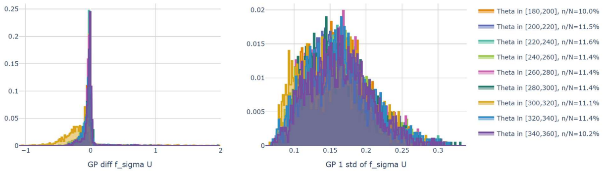
Figure 93 : Teesside: Histograms of \hat{f}_{\sigma_u}^{F-D}(\mathbf{x}) (left) and of its std (right). Each histogram is normalized by the number of observations of the \theta bin indicated by the color in the total LHS.
