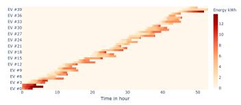
Fig. 1. Optimal energy time series for MPC simulation
