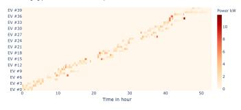
Fig. 3. Optimal charging time series for MPC simulation
