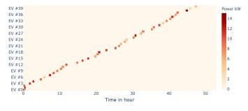
Fig. 4. Reference charging time series for MPC simulation
