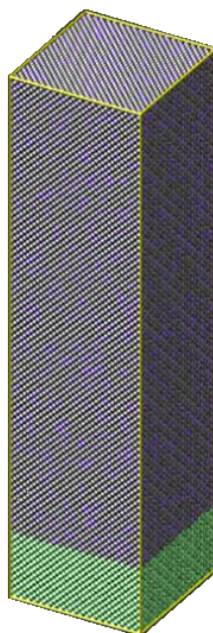
Figure S6: Simulation box size: 8.8 \text{ nm} \times 8.8 \text{ nm} \times 35.2 . the lower green box compartment represents Li-metal, and the upper compartment represents the bulk EC
