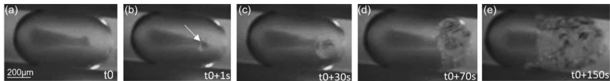
Figure 11. Example of progression of CPH crystallization in a pure water droplet – secondary CPH formation.
