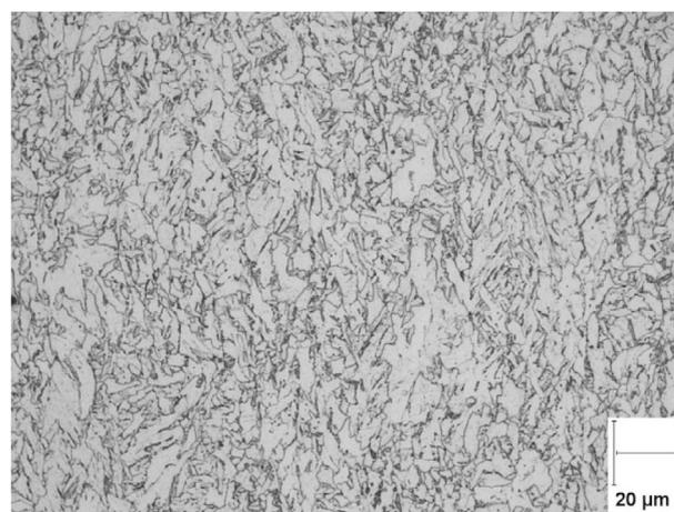
**Fig. 1 – Microstructure of the studied  $\times 65$  steel after Nital Etching.**
