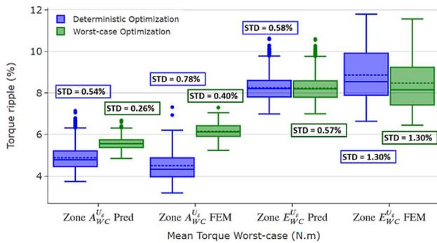
**Fig. 19.** Boxplots showing comparisons of torque ripple between FEM simulations and surrogate model predictions: deterministic (blue) and robust (green) machines with similar predicted mean torque worst-case values.
