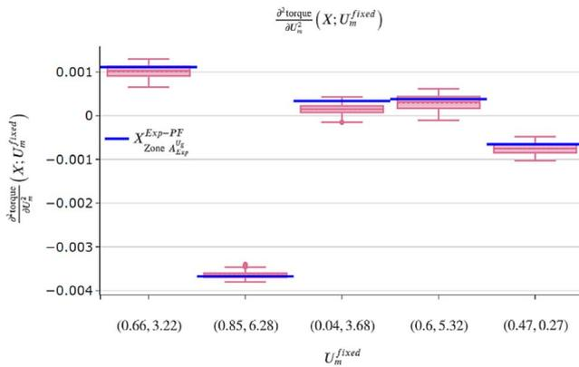
**Fig. 16.** Boxplots showing the variability (with respect to a batch of  $X_g$  samples) of the mean torque metamodel second partial derivative (with respect to  $U_m$ ) evaluated at a given value of  $U_m$ . The blue horizontal lines stand for the machine related to zone  $A_{Exp}^{Ug}$  and coming from the expectations Pareto front.
