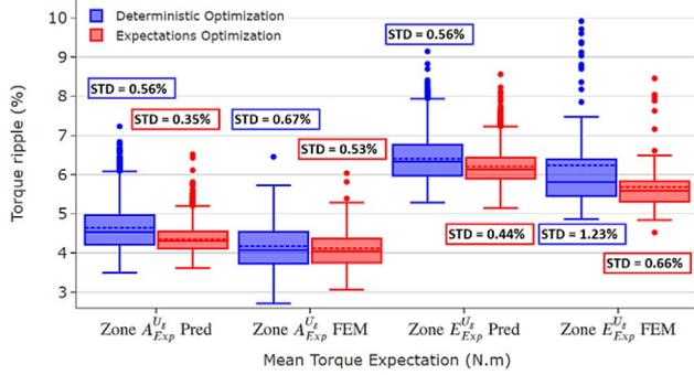
**Fig. 18.** Boxplots showing comparisons of torque ripple between FEM simulations and surrogate model predictions: deterministic (blue) and robust (red) machines with similar predicted mean torque/ mean torque expectation values.
