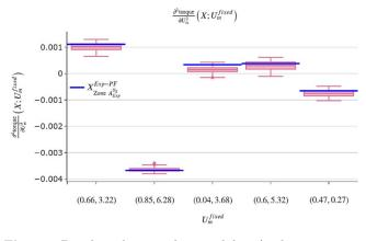
Fig. 16. Boxplots showing the variability (with respect to a batch of Xg samples) of the mean torque metamodel second partial derivative (with respect to Um) evaluated at a given value of Um. The blue horizontal lines stand for the machine related to zone  $A_{Exp}^{Ug}$  and coming from the expectations Pareto front.
