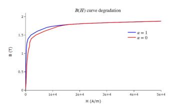
Fig. 4. Nominal and degraded B(H) curve.
