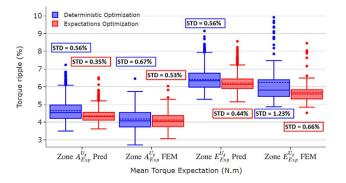
Fig. 18. Boxplots showing comparisons of torque ripple between FEM simulations and surrogate model predictions: deterministic (blue) and robust (red) machines with similar predicted mean torque/ mean torque expectation values.
