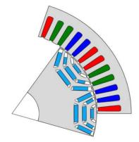
Fig. 1. Geometry of the PMaSynRelM motor.
