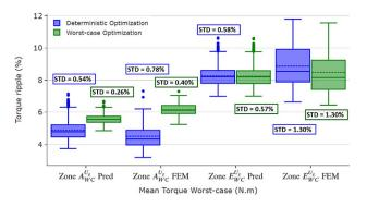
Fig. 19. Boxplots showing comparisons of torque ripple between FEM simulations and surrogate model predictions: deterministic (blue) and robust (green) machines with similar predicted mean torque worst-case values.
