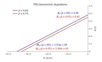
Fig. 3. Nominal and degraded PM characteristic.
