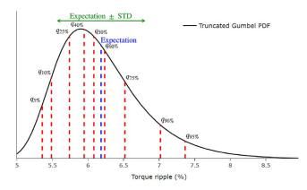
Fig. 8. Example of a torque ripple PDF.
