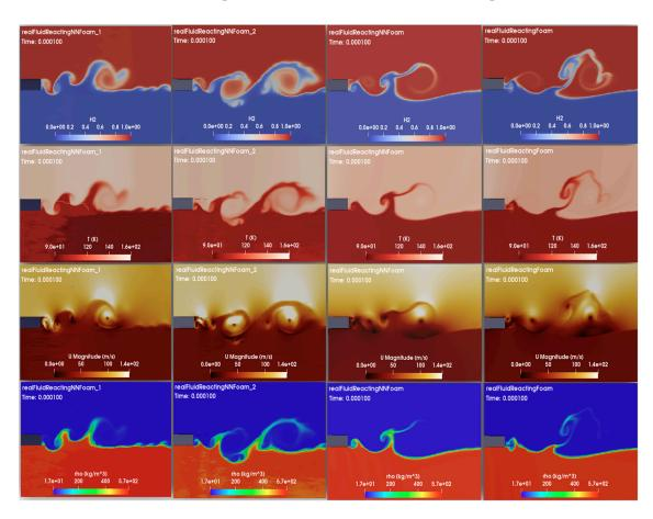
**Figure 10.** Instantaneous fields of  $H_2$  mass fraction, temperature, velocity magnitude, and density at 0.1 ms for realFluidReactingNNFoam\_1, realFluidReactingNNFoam\_2, realFluidReactingNNFoam, and realFluidReactingFoam solvers.
