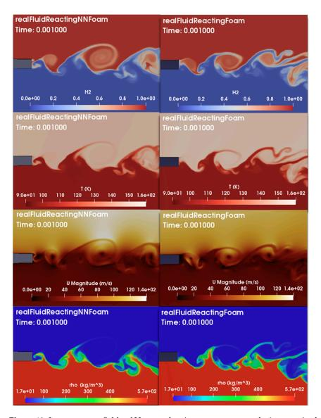
**Figure 12.** Instantaneous fields of  $H_2$  mass fraction, temperature, velocity magnitude, and density at 1 ms for realFluidReactingNNFoam and realFluidReactingFoam solvers.
