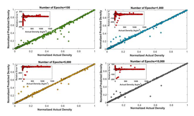
**Figure 3.** Representation of the effects of a higher number of epochs on network performance and the values of the relative error.
