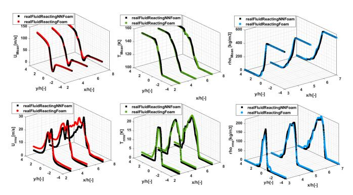
Figure 13. Transverse profiles of mean (up) and rms (down) x-velocity, temperature, and density.
