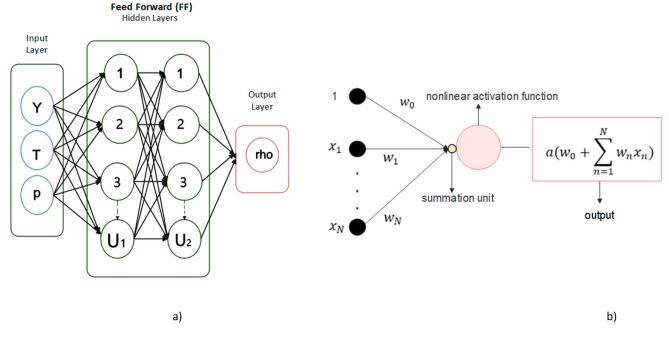
**Figure 1.** Schematics of NN with one input layer, two hidden layers, and one output layer with  $U_1$  and  $U_2$  numbers of units, or neurons (a), and typical structure of a neuron showing input weights, bias, and activation function (b).
