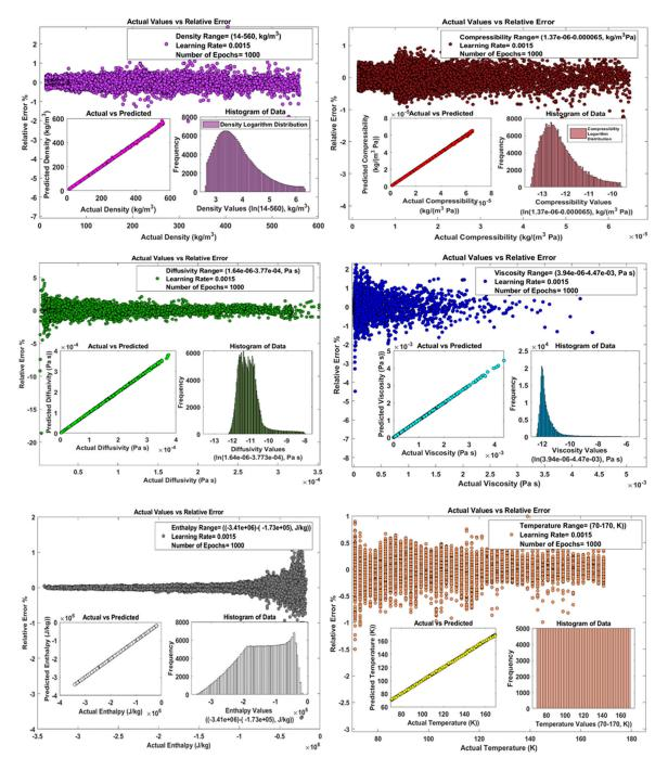
**Figure 7.** Representation of actual vs. predicted values, actual vs. relative error, and distribution of density (purple), compressibility (red), thermal diffusivity (green), viscosity (blue), enthalpy (gray), and temperature (orange). Adapted data range. T: 70-170 K;  $Y_{H2}: 0-1$ ; p: 50-150 bar (this model is referred to as NN variant, or final version, in Section 3).
