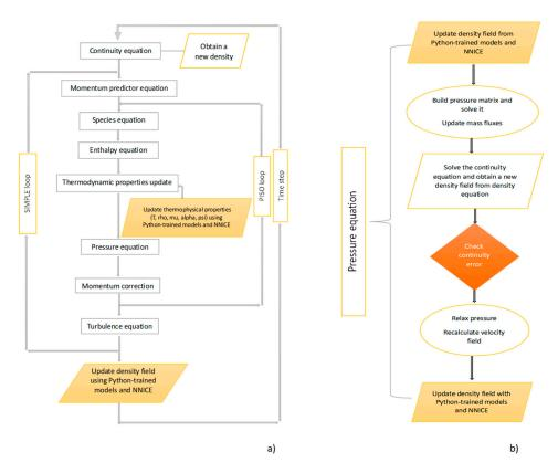
**Figure 8.** Extended PIMPLE solution flow chart for the multiphase transport equations with real-fluid properties (**a**) and pressure equation flow chart (**b**).
