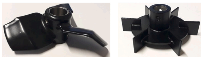
Fig. 1. HTPG4 impeller and Rushton turbine used in this study coated with black paint to minimize laser refraction.
