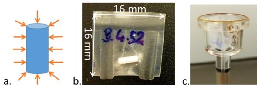
Figure A. 1: a) Schematic representation of the hydrostatic compression test (homogenous compression applied in all the directions. a) Example of extrudate within the waterproof membrane. c) cell recommended for the hydrostatic compression test with 1.6 cm of diameter
