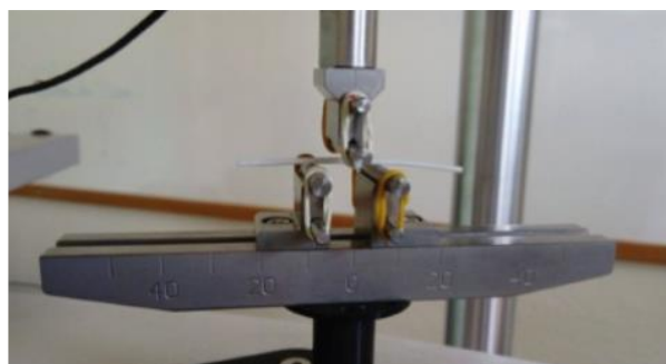
Figure 3.2: Three-point bending test performed on cylindrical support
